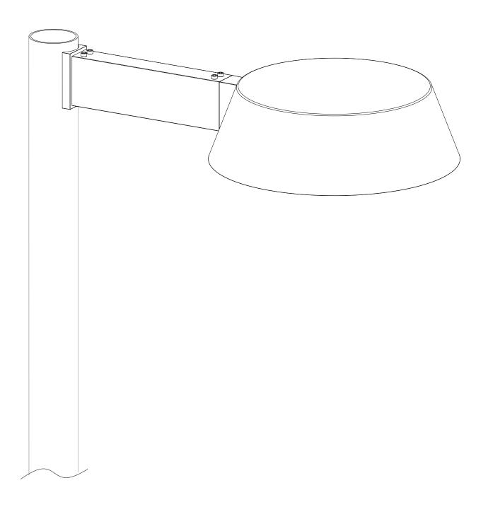
**Notes:** Do not energize luminaire until installation is completed. General contractor is responsible for providing appropriate anchoring devices to support load of fixture.
